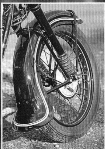
Front mudguard may look old-fashioned, but valance protects generator from spray.
