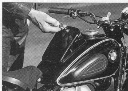
Toolbox is built into the top of the fuel tank.
